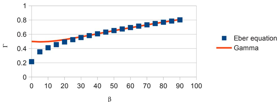
Even though it is not directly mentioned, Ebers model presumably covers the case of turbulent flow only. There is no reason to believe that the laminar flow Nusselt number model for flat plates should not apply also for cones, and the shape conversion should therefore apply for both flow regimes.
