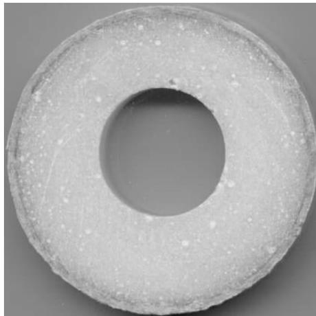
**Cut through propellant segment**
